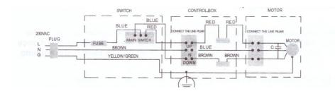
If the motorized screen work with remote control, please refer to the diagram below for electrical connection.
