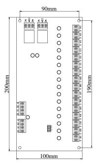
Z1, Z2: Connecting to the loop of control panel, non-polarized.
